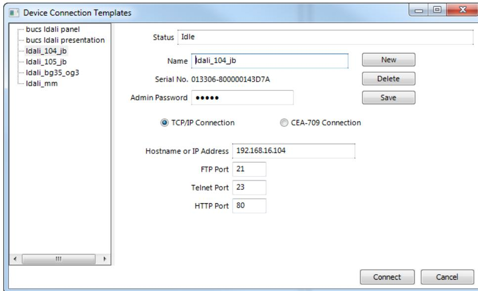
Figure 12: L-DALI Configuration Software, Connection Dialog
