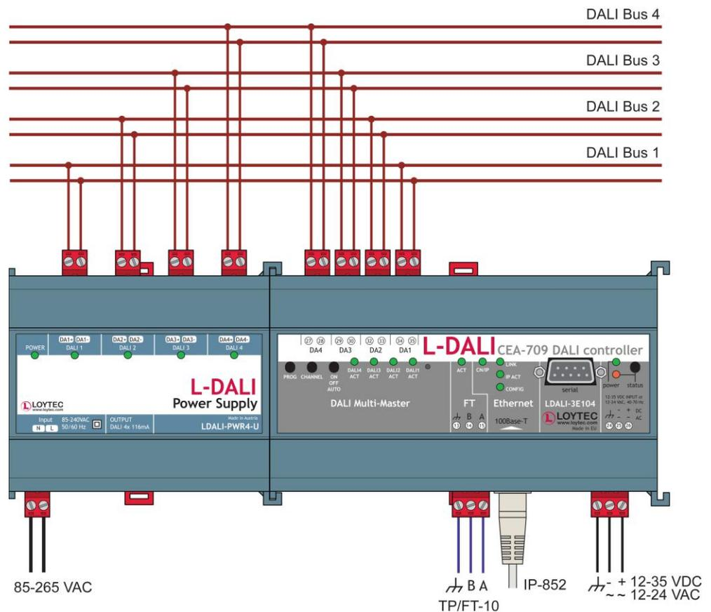
Figure 4: Basic Hardware Installation.
