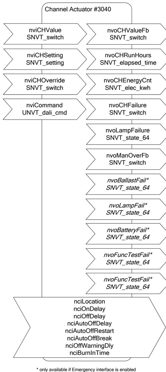
Figure 135: Object for channel
