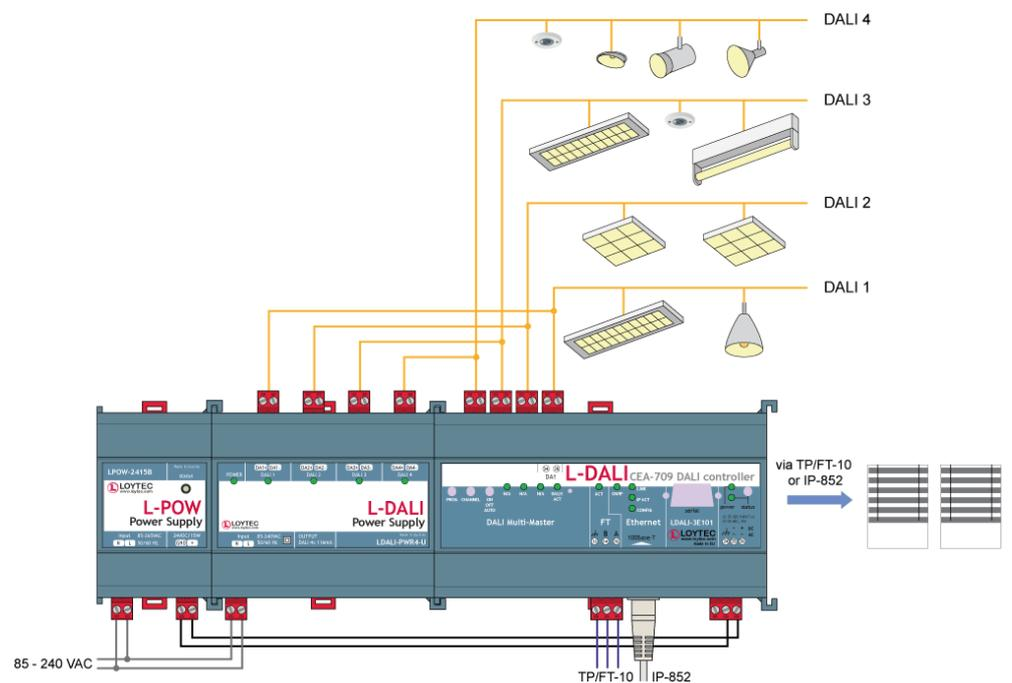
Figure 1: L-DALI supports up to four DALI channels
