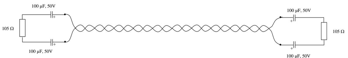
Figure 163: Termination in an FT Bus Topology
