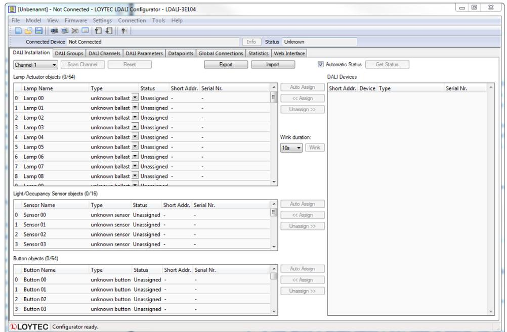
Figure 10: L-DALI Configuration Software, Start
