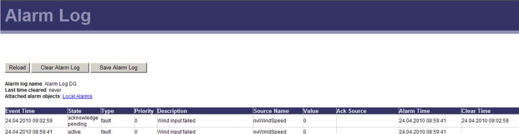
The screenshot shows the 'Alarm Log' page with a dark blue header. Below the header are three buttons: 'Reload', 'Clear Alarm Log', and 'Save Alarm Log'. Below the buttons, there is text indicating the alarm log name is 'Alarm Log DG', the last time cleared is 'never', and the attached alarm objects are 'Local Alarms'. A table follows with columns for Event Time, State, Type, Priority, Description, Source Name, Value, Ack Source, Alarm Time, and Clear Time. The table contains two rows of data.
