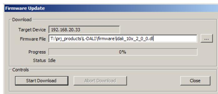
Figure 165: Firmware Update dialog of the LDALI Configurator.
