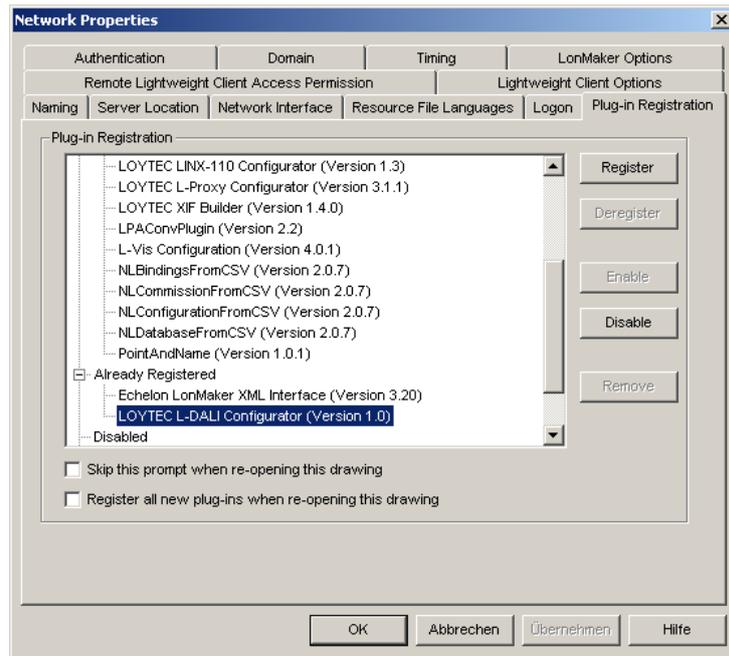
Figure 82: Check that the LDALI Configurator is properly registered.
