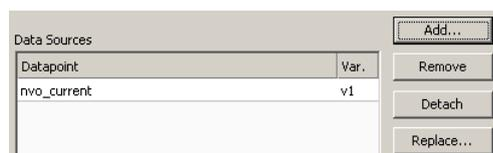
7. Select the data point in the **Data Sources** list. In the drop-down box underneath select **Selected Data Source Value** and click the **Paste to Text** button.
