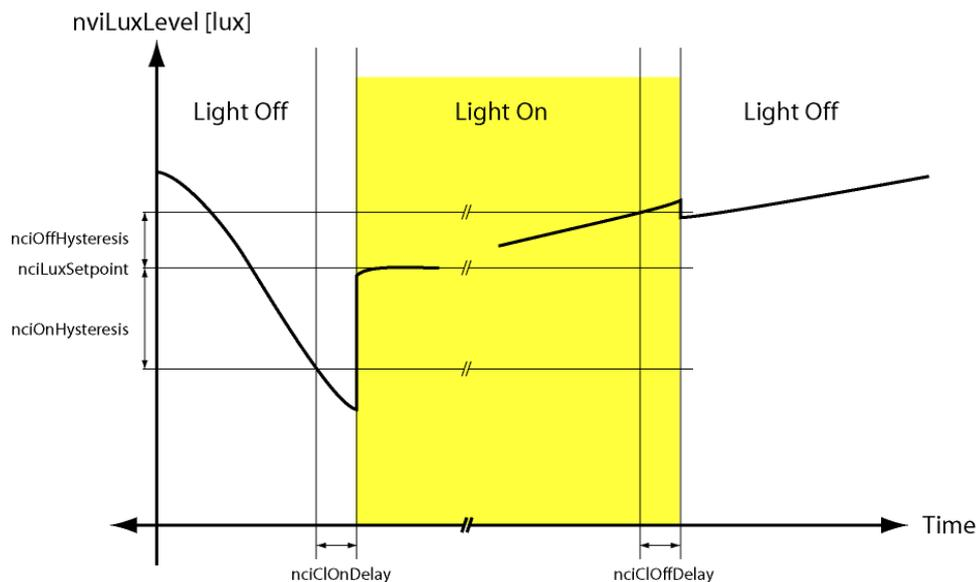
Figure 148: Constant Light Controller Timing
