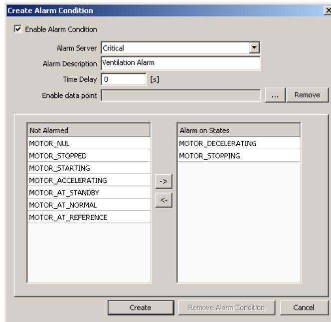
Figure 126: Alarm Condition for a Multi-State Data Point.
