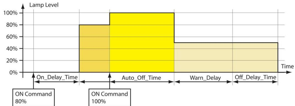
Figure 156: Timing Parameters (restart enabled).
