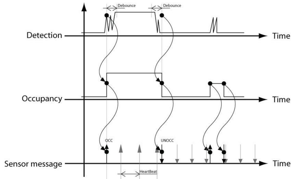
Figure 143: Timing of occupancy detection.
