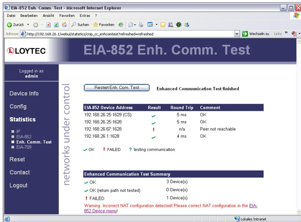
Figure 71: Enhanced Communication Test Output
