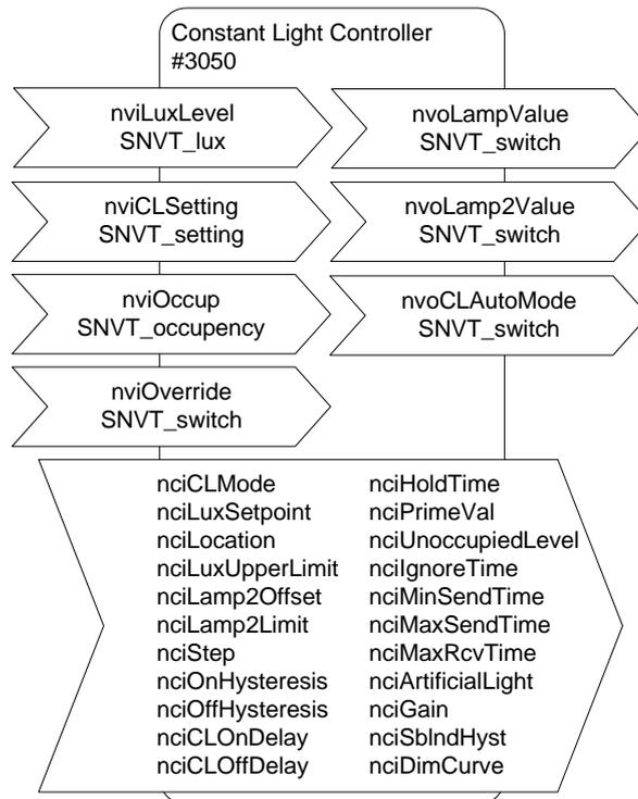
Figure 144: Constant Light Controller Object
