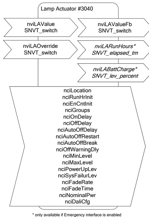
Figure 133: Lamp Actuator Object
