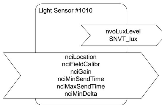
Figure 141: Light Sensor Object
