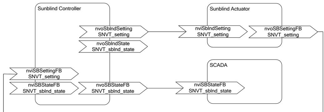
Figure 152: Controlling a Sunblind Actuator via *SNVT\_setting*
