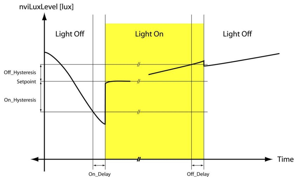
Figure 158: Constant Light Controller Timing.
