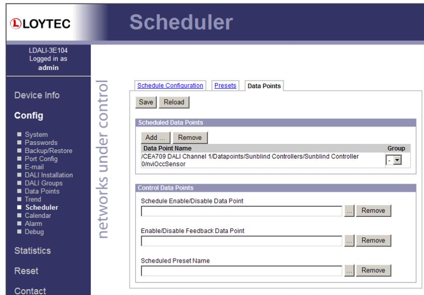
Figure 63: Re-configure scheduled data points on the Web UI.
