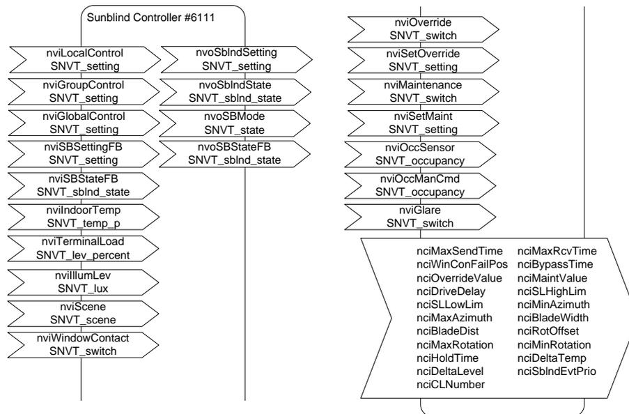
Figure 149: Sunblind Controller Object
