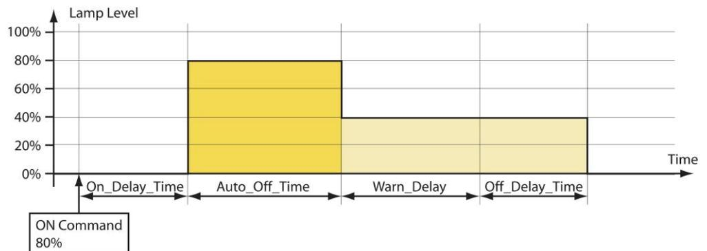
Figure 155: Timing Parameters with *Auto\_Off\_Time* and *Warn\_Delay*.
