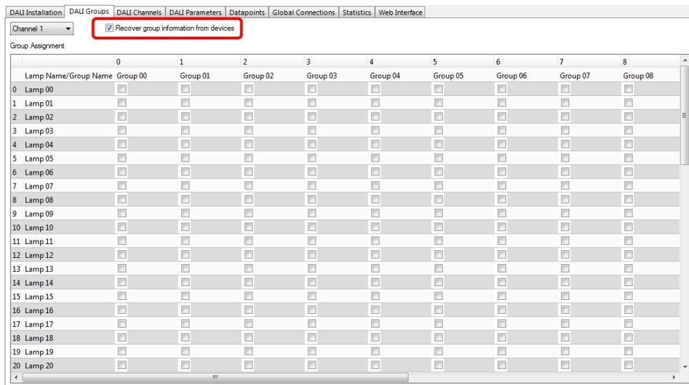
Figure 161: Be sure to check the **Recover group information from devices** checkbox if group addresses were already assigned with the IRT 8099/10 omniprogram.
