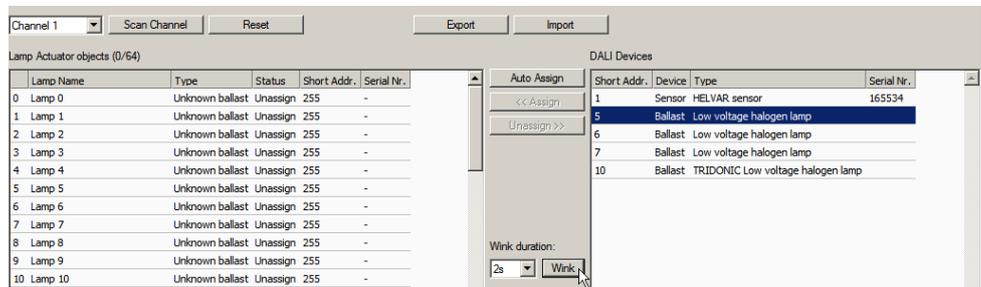
Figure 15: L-DALI Configuration Software, Wink Button
