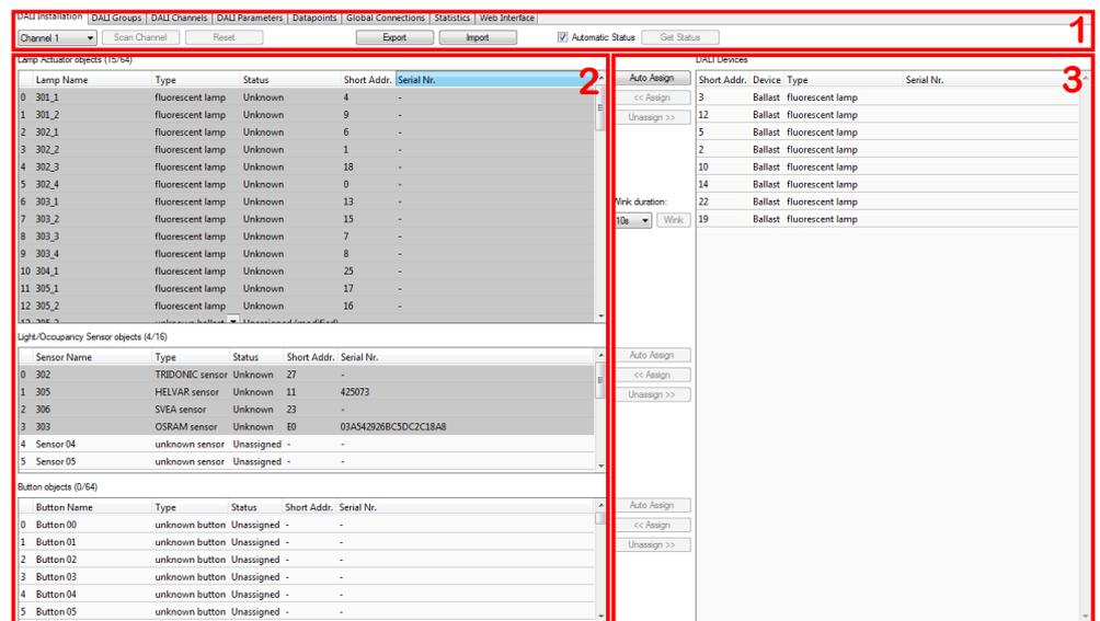
Figure 106: DALI Installation tab.
