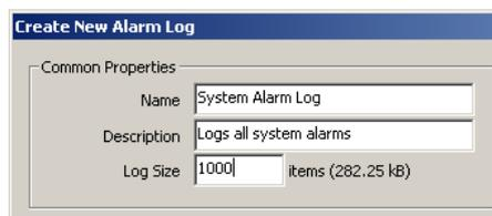
3. In the **Create New Alarm Log** dialog enter a **Name** for the alarm log. Optionally enter a **Description**.
