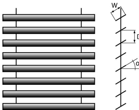
Figure 150: Sunblind Geometry
