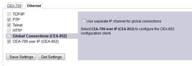
Figure 45: Global Connections Configuration Page.
