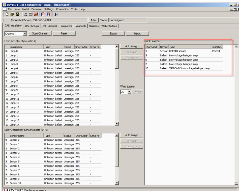
Figure 14: L-DALI Configuration Software, Detected DALI Devices
