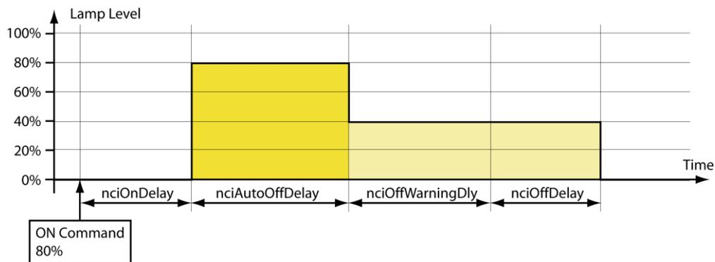
Figure 137: Timing Parameters with *nciAutoOffDelay* and *nciOffWarningDly*
