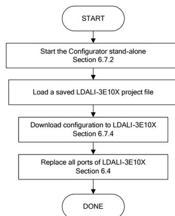
Figure 85: Basic work flow to configure a replacement device.
