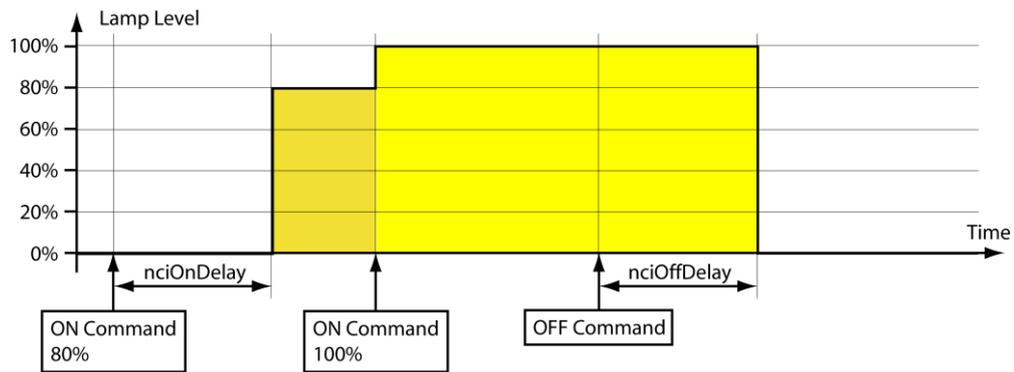
Figure 136: Timing Parameters
