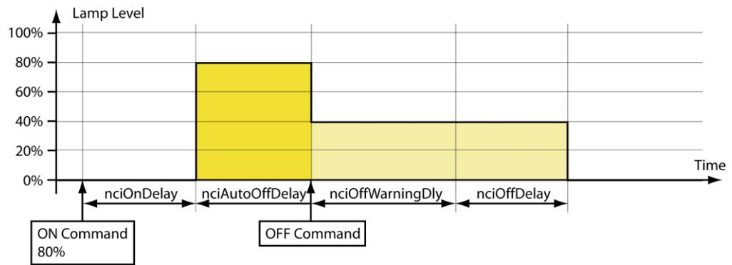
Figure 139: Timing Parameters (*nciAutoOffBreak=ST\_ON*)
