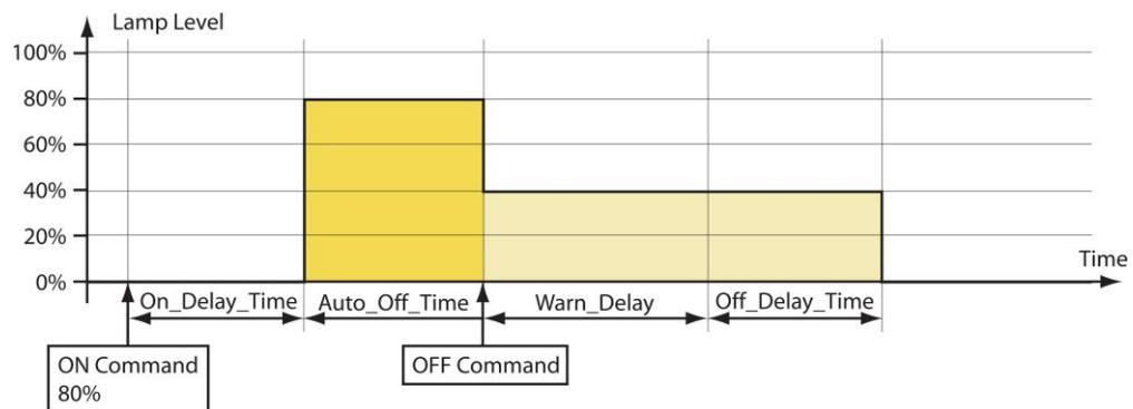
Figure 157: Timing Parameters (break enabled).
