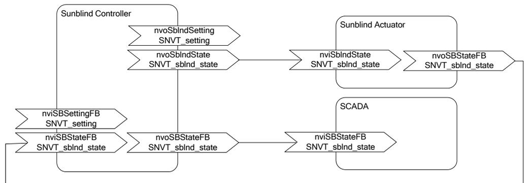
Figure 151: Controlling a Sunblind Actuator via *SNVT\_sbld\_state*
