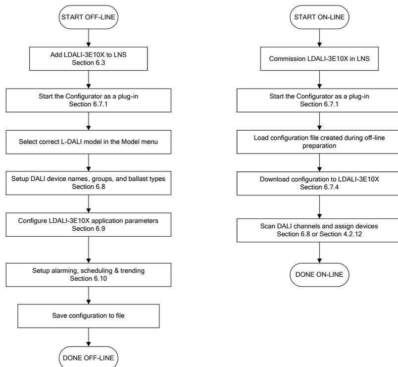
Figure 84: Basic off-line design-flow.
