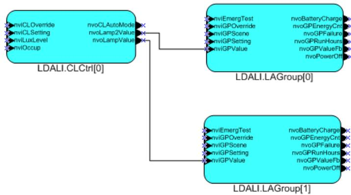
Figure 31: Network Variable Bindings
